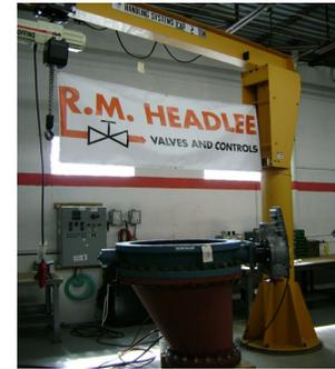
Buffalo Sewer Authority wanted to replace (2) 36" and (2) 24" glued-in "Seat-In Body" design AWWA butterfly valves with a seat design to allow for field reparability should the need arise. The Val-Matic American Butterfly Valve was chosen for the cost effectiveness and operational flexibility advantages over the glued-in "seat-in-body" designs. Val-Matic's Tri-Loc seat retention system provides positive mechanical retention of the valve seat while allowing easy adjustment and replacement.
